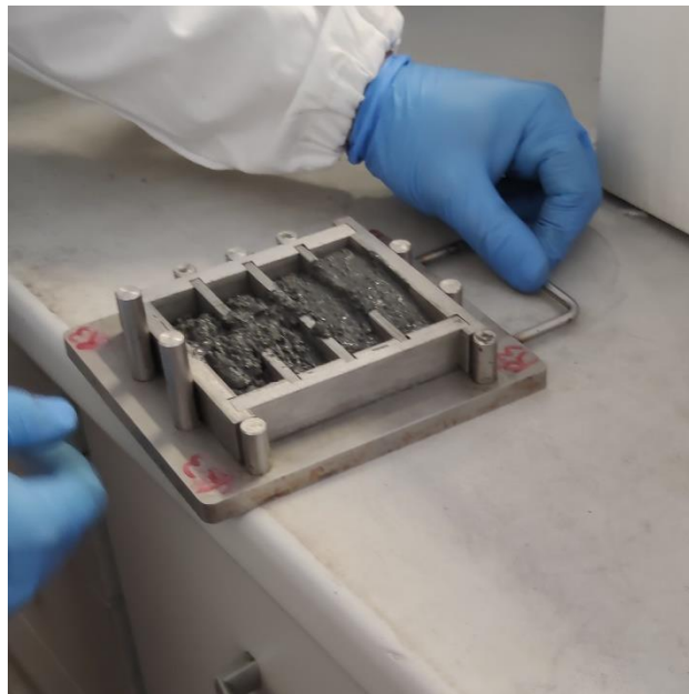
Figure 3. Taping molds 30 times for precise air bubbles removal.
