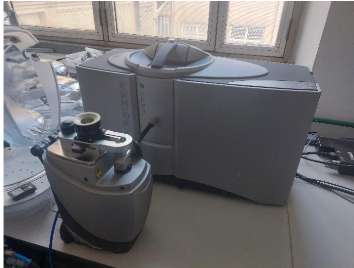
Figure 6. Granulometric analysis with Mastersizer 3000.
