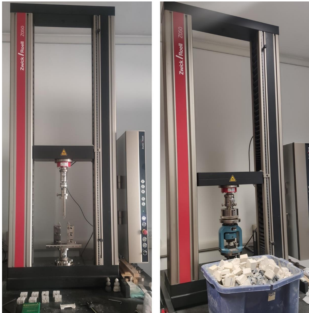
Figure 5. Zwick/Roell mechanical for flexural (left) and compression (Right) strength.
