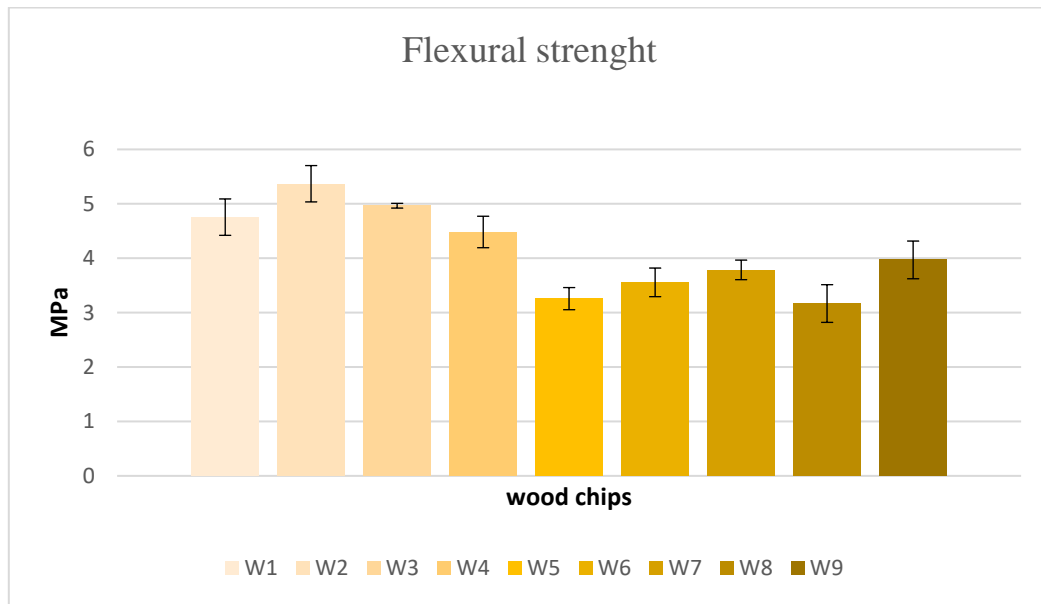
Figure 21. Displays measurements from W1 to W9 of wood chips substitution on material performance in flexural tests.
