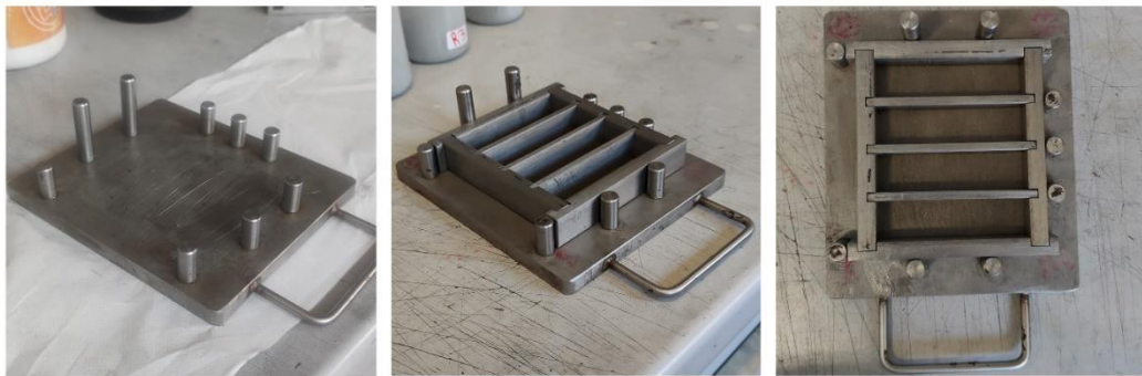
Figure 1. Sample frames with greasing are used in mortar testing.
